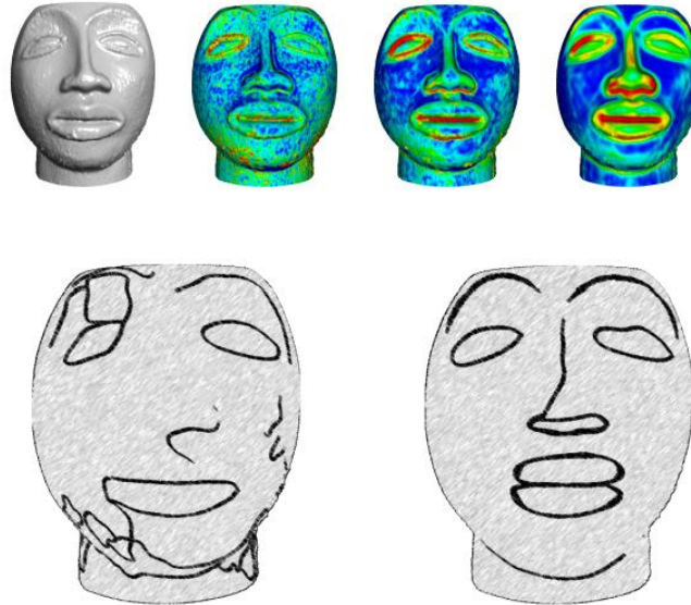
Figure 34. Multi-scale feature extraction (bottom right) is superior to single scale extraction (bottom left) on a noisy range scan. The top row shows the original point cloud and variation estimates for different scales.
