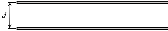
Figure 21.6. Isolated two-wire electric power transmission line
