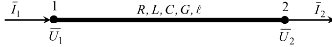
Figure 21.9. Simplified representation of electric voltages and currents in a two-wire transmission line
