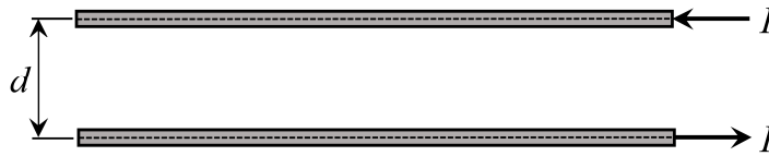
Figure 16.63. Two-wire isolated electric line
