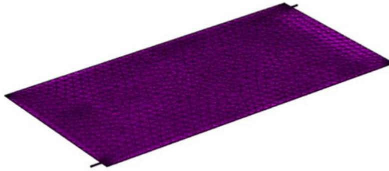
*Fig. 5.1. Unstructured finite element mesh of PVT-PCM collector concept, [30].*
